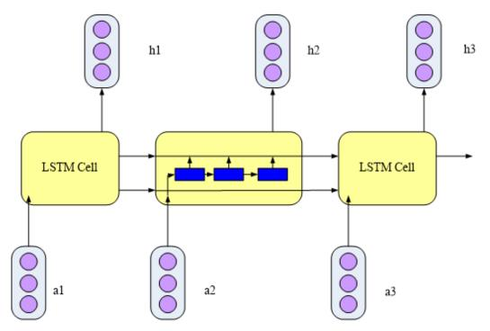
As shown in Figure 3, the output of the first layer of LSTM neurons is transmitted to the next layer of LSTM neuron memory, and it is also transmitted to itself and the same layer of neuron memory blocks (Lu et al.,2020).
